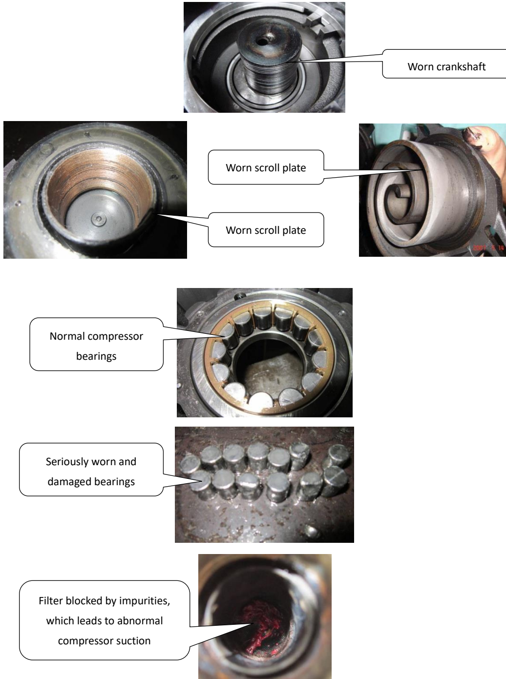
Figure 6-2.11: Effects of spoiled compressor oil
