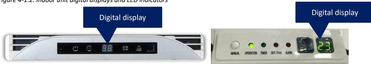
Figure 4-1.2: Indoor unit digital displays and LED indicators
