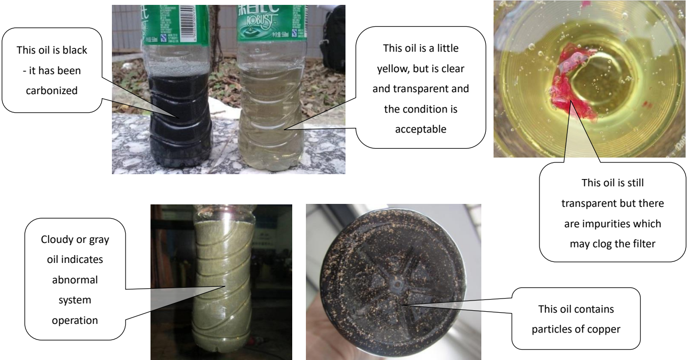
Figure 6-2.10: Inspecting compressor oil
