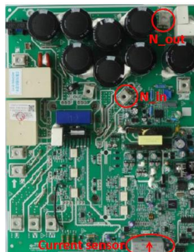
Figure 6-2.5: DC detection wire connection method
