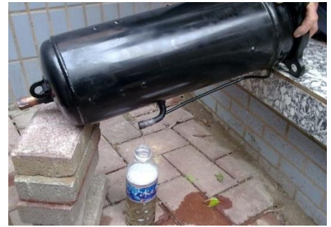
Figure 6-2.8: Draining oil from a compressor
