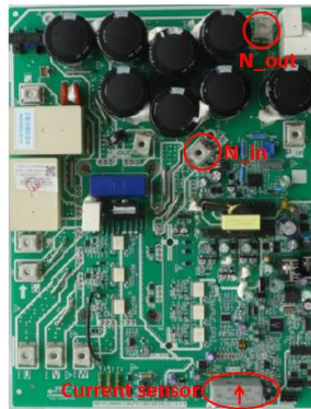
Figure 6-2.2: DC detection wire connection method
